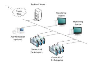
Picture 10. Autogate System Network
